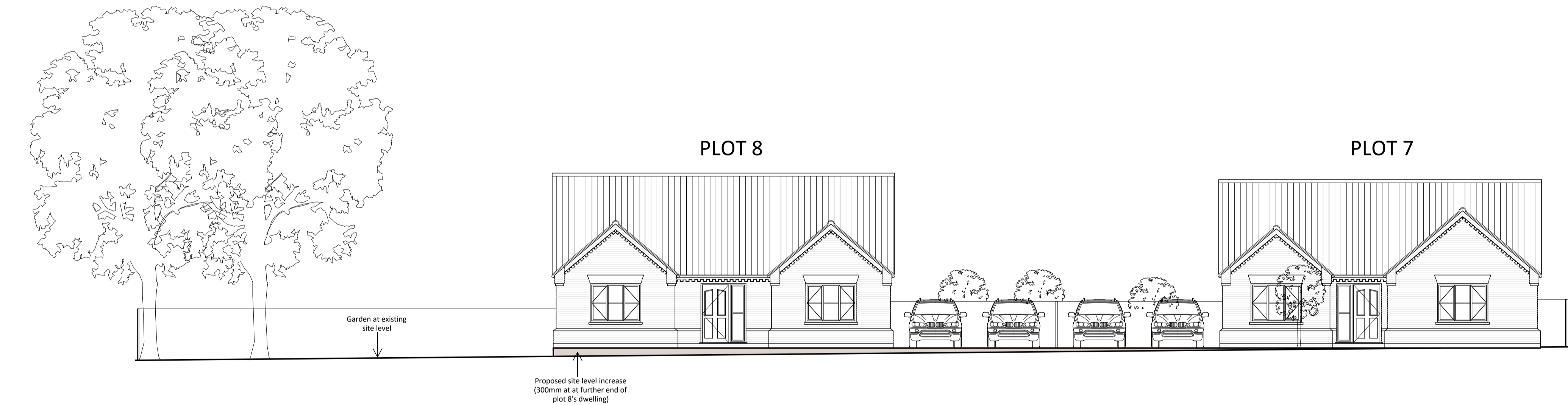
PROPOSED LONG SECTION AT PLOT 8 1:100 (SHOWING LAND LEVEL INCREASE TO PLOT 8)
